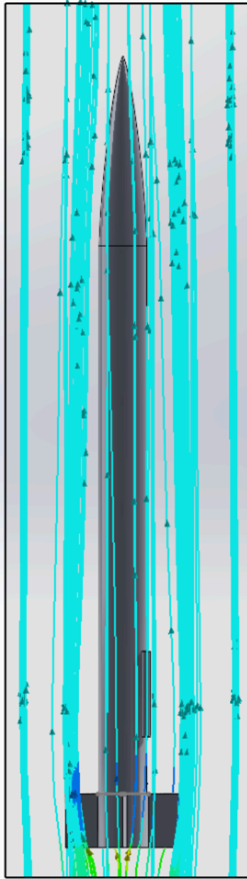
Figure 4: Qualitative flow and pressure visualization around the rocket geometry. Cooler colors indicate lower displayed pressure and warmer colors indicate higher displayed pressure.
